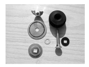
Make sure that you examine your test plug. It should be the rubber type, not plastic. Some of them come with a washer on top that is larger than 2". Replace it with one that is 11/2" in diameter that has a 3/8" hole and is of the same thickness.
