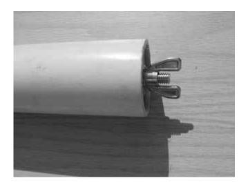
7. Use the wingnut to adjust the plug so it makes a good seal yet allows the handle and rod to be pumped up and down smoothly. Adjust the plug once you're in the field. Thick sand, mud or lack of water may require you to loosen and retest the plug.
