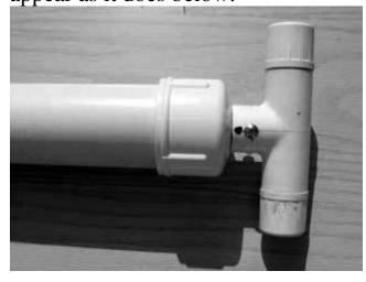
Note: You can make this pump WITHOUT the caps and WITHOUT the screw and WITHOUT the 1/2" reinforcement... (Just glue the t-handle to the top of the 36" piece of 3/4" PVC)
